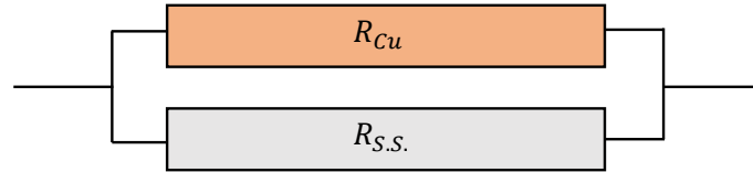
Figure 2.21: Schematic representation of the septum's blade resistance.
