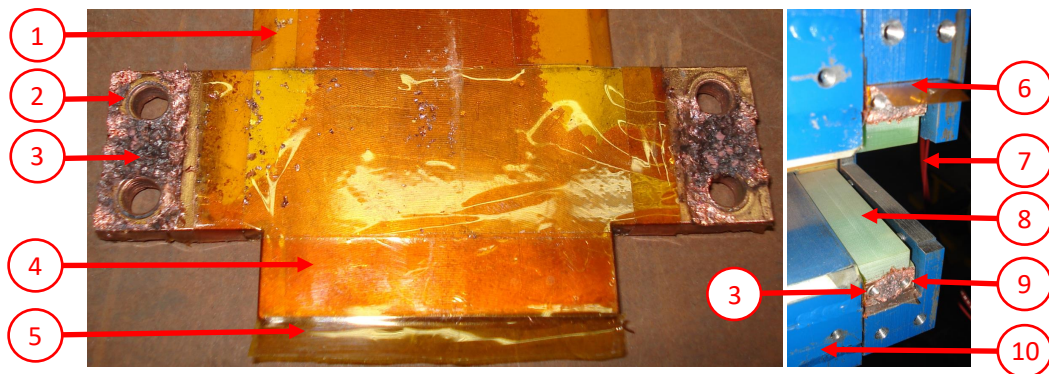
Figure 3.5: Two photographs of a failure that occurred in 2012 as a result of not sufficiently tightening the coil fasteners [32].
