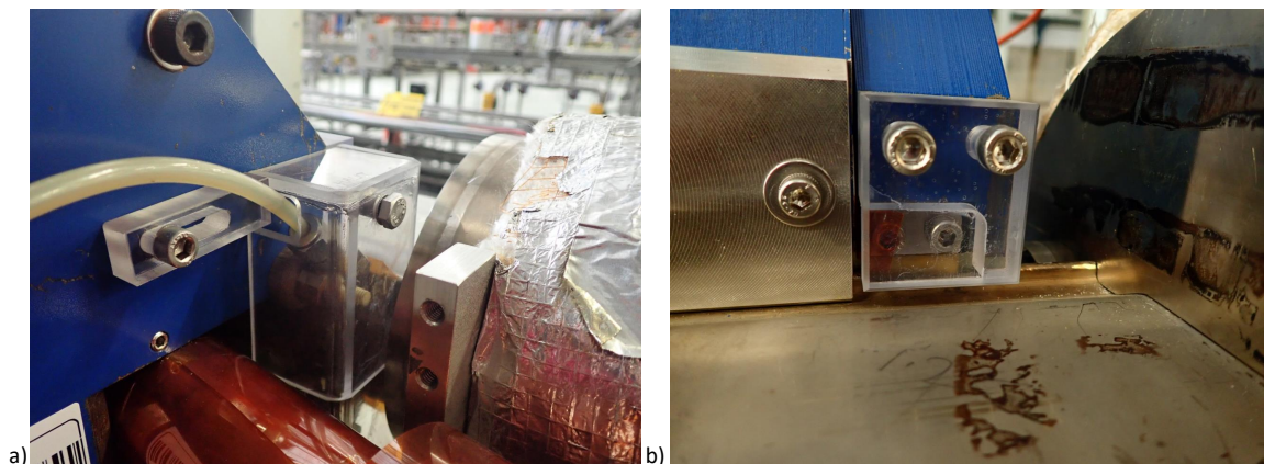
Figure 2.11: a) Photograph of the safety cover on the water block. Photograph of the removed cover is shown in Figure 2.7 b) One out of four covers for the mounting areas.
