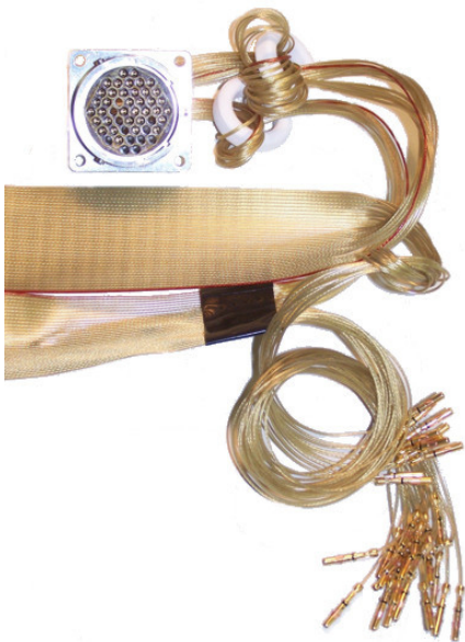
Figure 10.12: Cable used for the pinout assignment between the long cable and the motherboard
