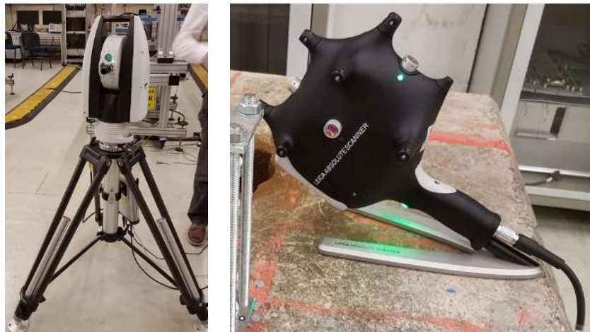
Figure 5.9 Specimen scanning with Leica ® LAS device. Left: tracking tripod. Right: Scanning handle.
