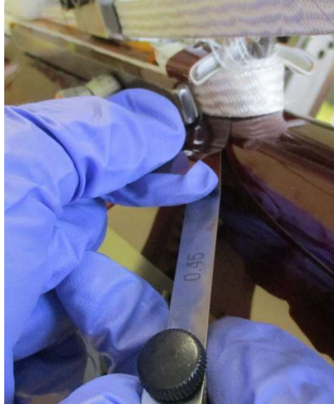
Figure 8.3 Protrusion measurement during winding with the wedge gauge of 50 \mu\text{m} resolution.
