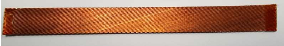
Figure 5.2 The undeformed thermography specimen, 150 mm-long uninsulated Nb 3 Sn cable.
