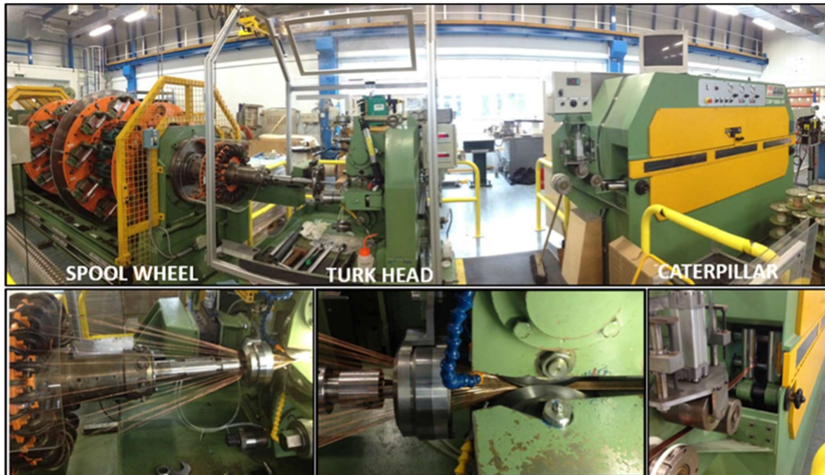
Figure 1.20 Cabling machine at CERN. Three sub-assemblies visible: spool wheel, Turk Head and caterpillar. Courtesy of CERN Superconducting Lab [45].
