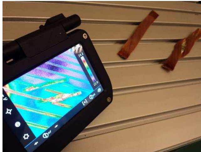
Figure 5.3 Uninsulated cable specimens, thermal reflex visible on LCD screen in red and white.
