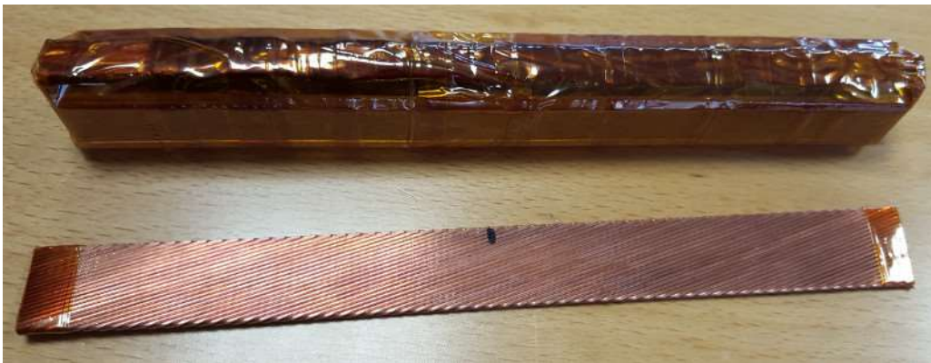
Figure 4.7 Specimens of 40-strand Nb 3 Sn 132/169 cable prepared for X-ray absorption tomography. Top: Sample B, a stack of four cables (18 mm x 12 mm x 150 mm). Bottom: Sample A, a single cable (15 mm x 2 mm x 150 mm).
