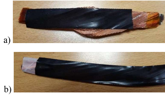
Figure 5.4 The tape-insulated specimens. a) sample A, strongly deformed; b) sample B, slightly deformed.
