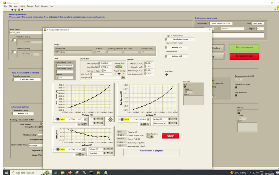
Figure 9: Labview software screenshot while running an IV measurement
