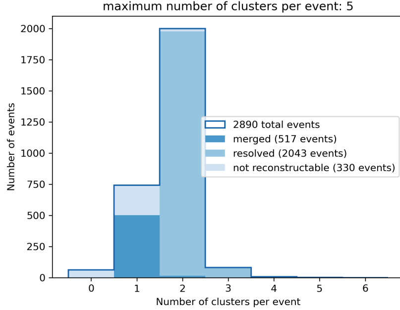
Figure 3: Number of clusters per \pi^0 event in the detailed LHCb Run 4 simulations.
