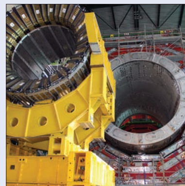
The first half of the barrel hadron calorimeter was tested in March 2006 using a radioactive source before insertion into the solenoid in early April. The second half was inserted a month later.
