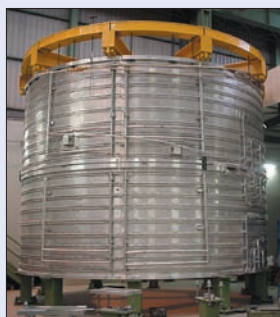
Two modules of the CMS solenoid at the manufacturers, Ansaldo, in Italy. The lower module was the first travel to CERN from Genova, at the end of January 2004. (Courtesy INFN.)
