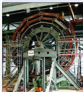
The first ring for the barrel yoke of the CMS superconducting magnet under assembly in 1999 by the manufacturer Deggendorfer Werft und Eisenbau GmbH (DWE) in Germany.
