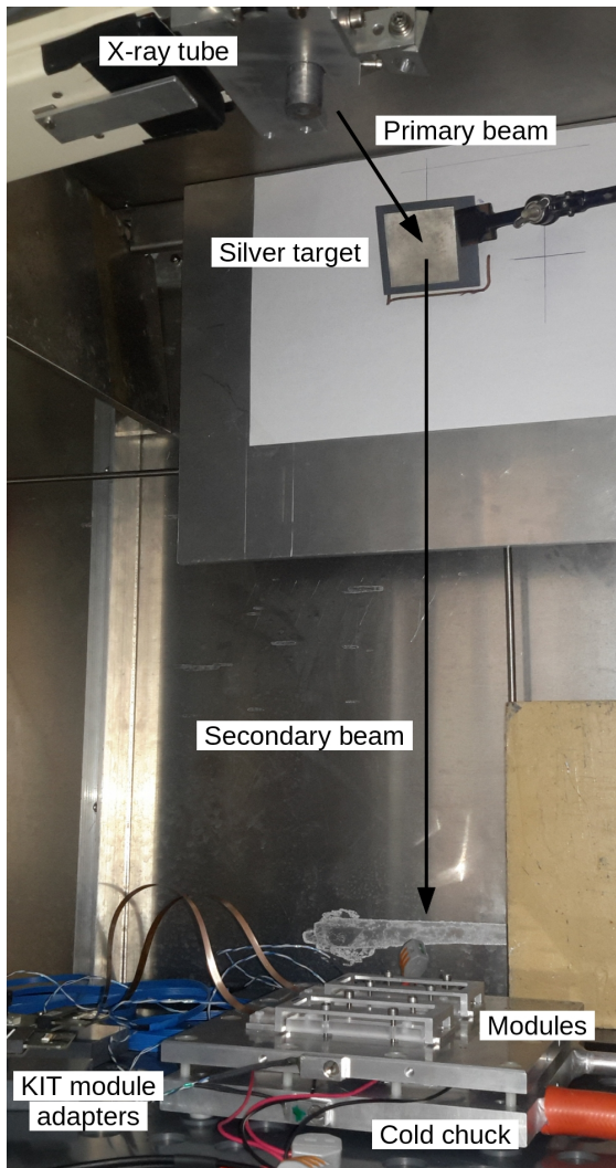
Figure 7.4: X-ray setup used for irradiation of modules produced at KIT. The backward-facing primary beam of the X-ray tube is used to create a secondary beam of characteristic X-rays by illuminating the silver target. The modules are placed on the cold chuck on the bottom of the shielding box and get irradiated by the secondary beam.
