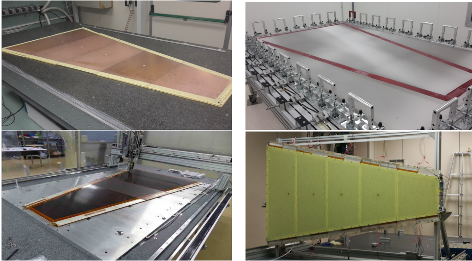
Figure 4.5. Top left: drift panel construction in Rome1. Top right: mesh stretching in Roma3. Bottom left: read-out panel construction in Pavia. Bottom right: final assembly of the module in Frascati.
