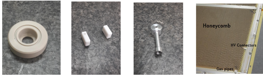
Figure 4.16. From left to right: the interconnections, HV connector, gas pipe used for the drift panel construction; the PCB1 during the construction phase, the position inside the panel of the honeycomb cutted sheet, the HV connectors and the gas pipes is shown.
