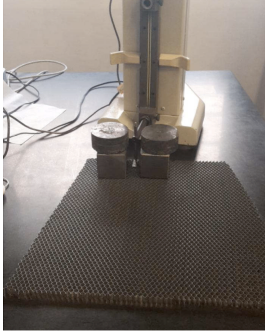
Figure 4.13. Mitutoyo Linear Height 600 during a honeycomb thickness measurement. Over the honeycomb cut sheet have been placed some weights (lead) to prevent the bending of the sheet.
