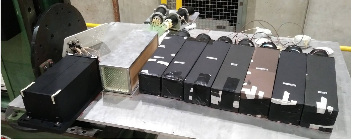
Figure 3.19: Photo of the calorimeters employed on the H2 line. From left to right: the photon calorimeter ( \gamma CAL), the shashlik calorimeter and the seven Lead Glass calorimeters (eCAL).
