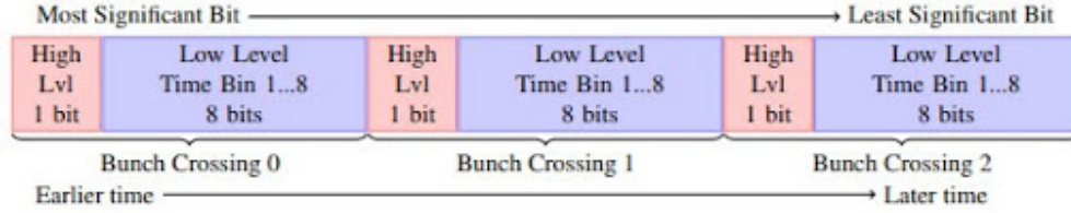
Figure 3.1: Structure of the 27-bit straw word. For Run 2 the last 4 bits were dropped giving a 23-bit word.
