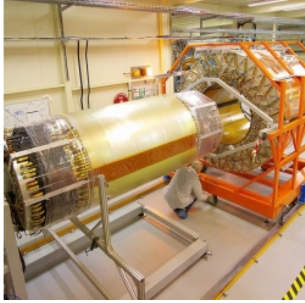
Figure 2.7: A picture showing both the SCT and TRT during production when the SCT is being placed in the center of the TRT.
