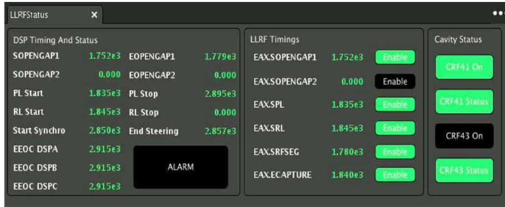
Figure 4.6: A screenshot of the LEIR LLRF diagnostic panel, fed by information coming from PyDAQ.
