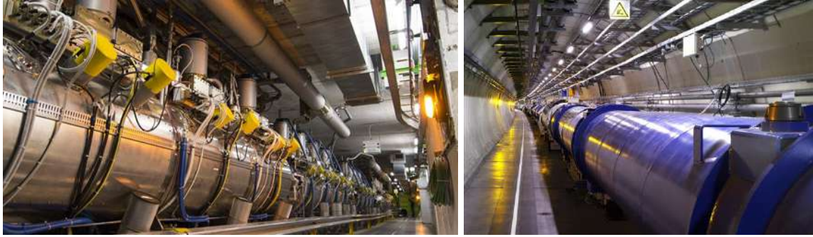
Figure 1.6: On the left is shown an LHC module containing RF cavities, on the right is shown a cryogenic dipole in the LHC
