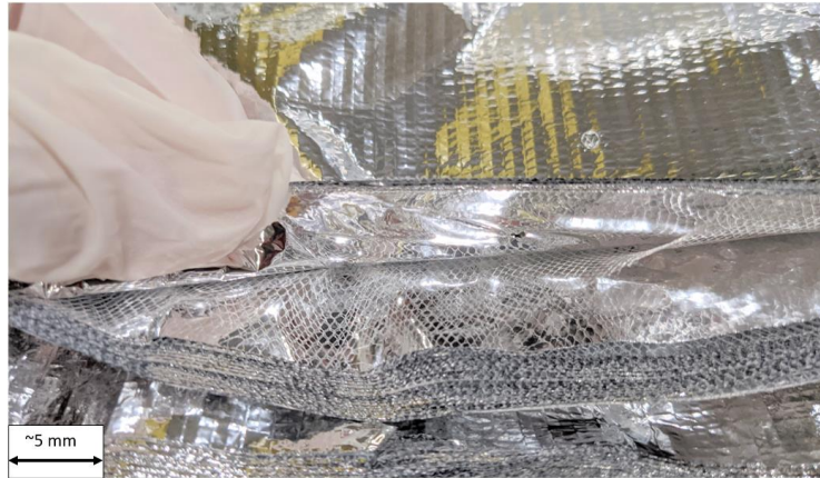
Figure 3.5. Multi-layer insulation foils of the ALPHA-g cryostat with 30 layers produced by HUTCHINSON®.
