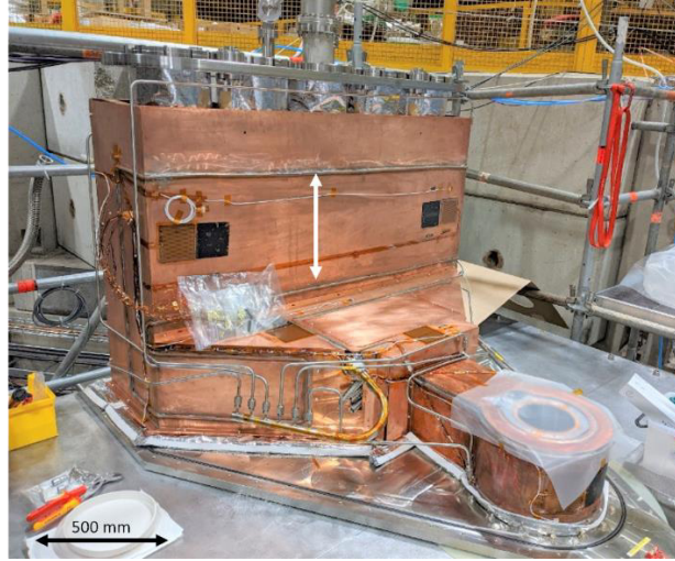
Figure 3.2. Copper shields of the upper part of ALPHA-g before the installation of the OVC box in May 2021. The gas distribution system from the shield tubes to the copper shields are visible.
