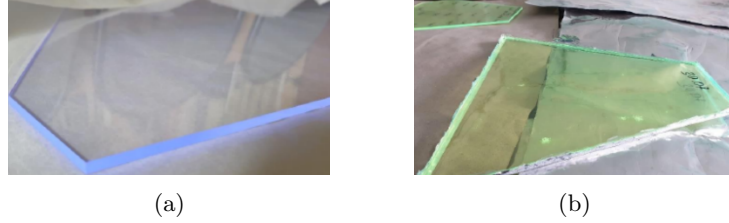
Figure 3: MBTS scintillators. (a) standard blue scintillator, (b) radiation-hard green scintillator
