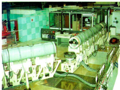
SOLENOIDS FOR NEUTRON SPIN ECHO SPECTROMETER (LLB CEA/CNRS).
