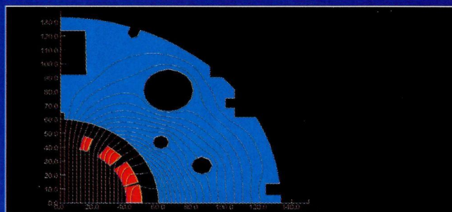
Flux lines for a typical dipole magnet.
