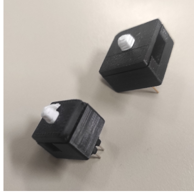
Figure 8.4: BaF 2 samples and their SiPM kept in place within black 3D-printed plastic holders. The detector on top, whose holder houses a Teflon-wrapped 3 \times 3 \times 10 mm 3 sample coupled to a 6 \times 6 mm 2 SiPM, was measured in the 2022 testbeam, while the one on the bottom was tested in 2023 and is composed of a 2 \times 2 \times 10 mm 3 crystal coupled to a 3 \times 3 mm 2 SiPM.
