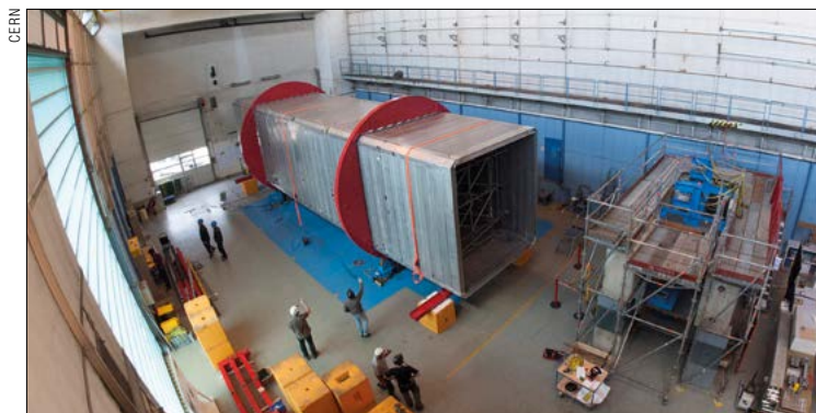
The ICARUS detector, formerly located at Gran Sasso National Laboratory, is being refitted at CERN before being shipped to the US to form part of Fermilab's short-baseline neutrino facility.
