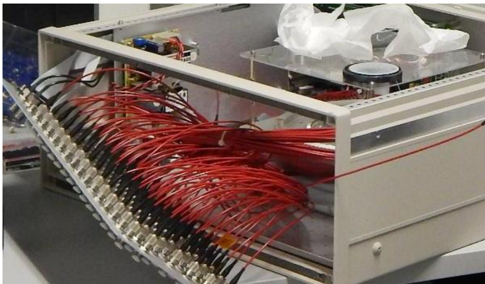
Figure 4.22: The view inside of the Switch 1x88. Its fibres were cleaned and polished before installation.
