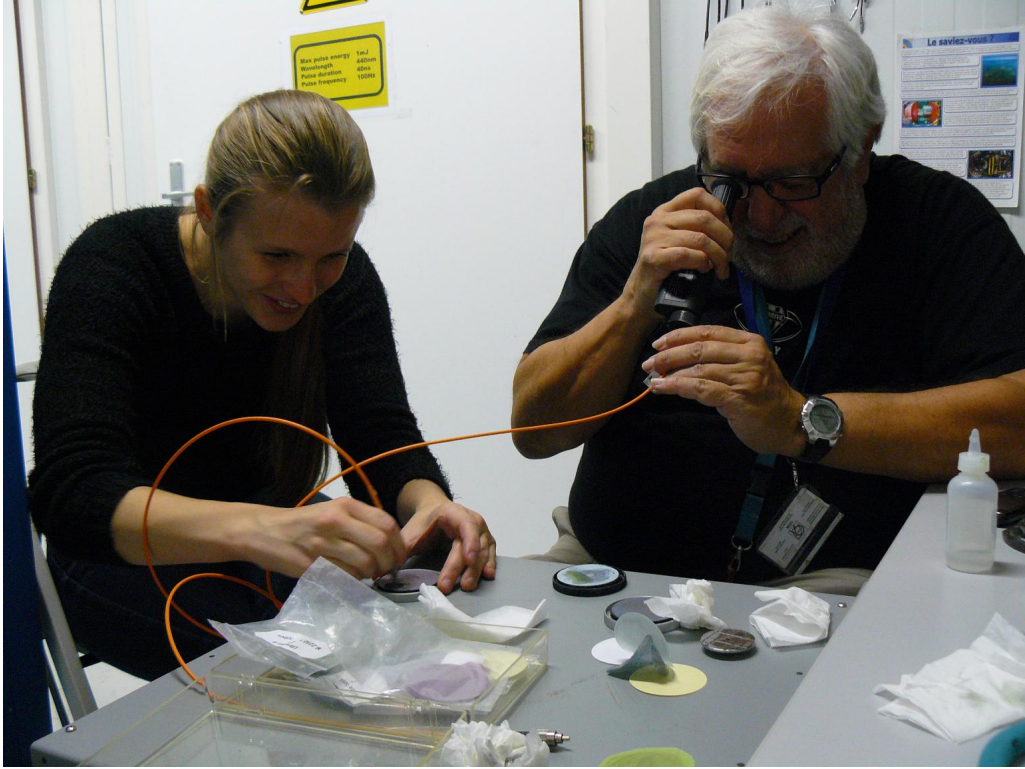
Figure 4.20: "SpyBox" fibres were cleaned and polished before installation.
