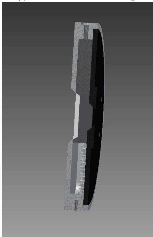
(b) Crosssection view on the first shutter design.
