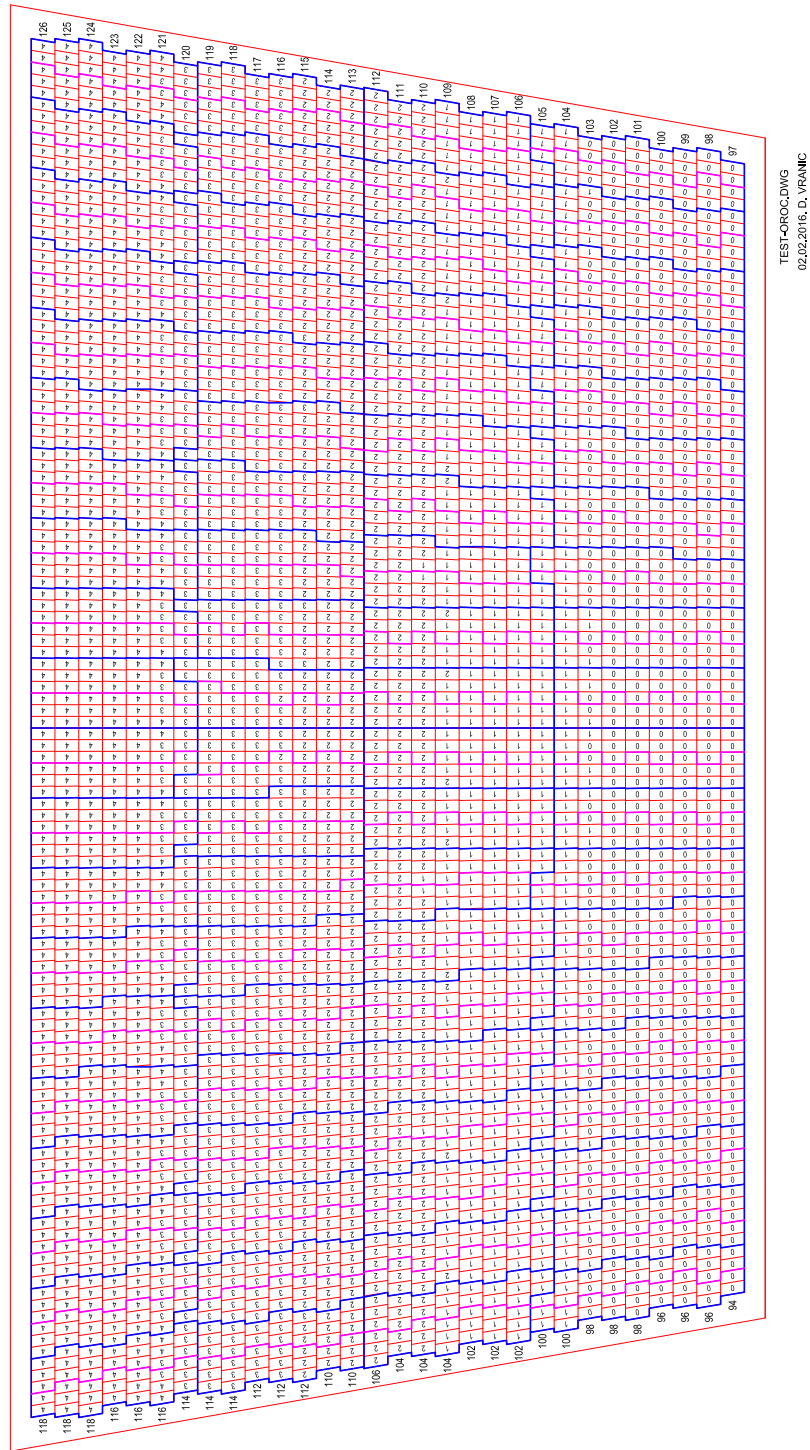
Figure B.3: The pad plane of the OROC 2. Each pad shows the ID of the SAMPA within a FEC to which it is connected to, taken from [34].
