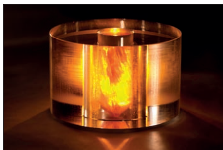
This maser core was developed at the National Physical Laboratory in the UK. (Image credit: Andrew Brookes/NPL.)
