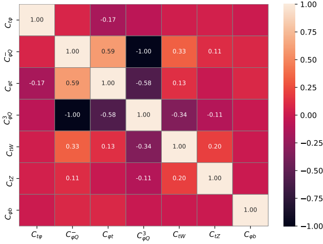
Figure A.5: Correlation matrix between the different EFT operators obtained in the linear ( \Lambda^{-2} ) “All correlations” robustness test fit described in Section 4.6.2. Cells are filled if the correlation is higher than 10% in absolute value. The operator O_{\varphi b} , that modifies only the bottom quark electro-weak couplings, is taken into account in the fit but limits on its coefficients are not reported since the obtained values are not competitive using only the observables considered in the fit.
