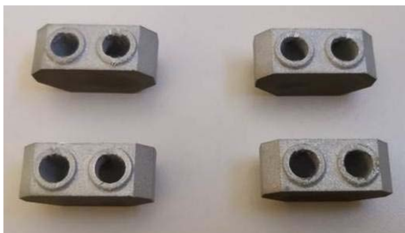
Figure 3.76 SLS 3D printed water returned clamps
