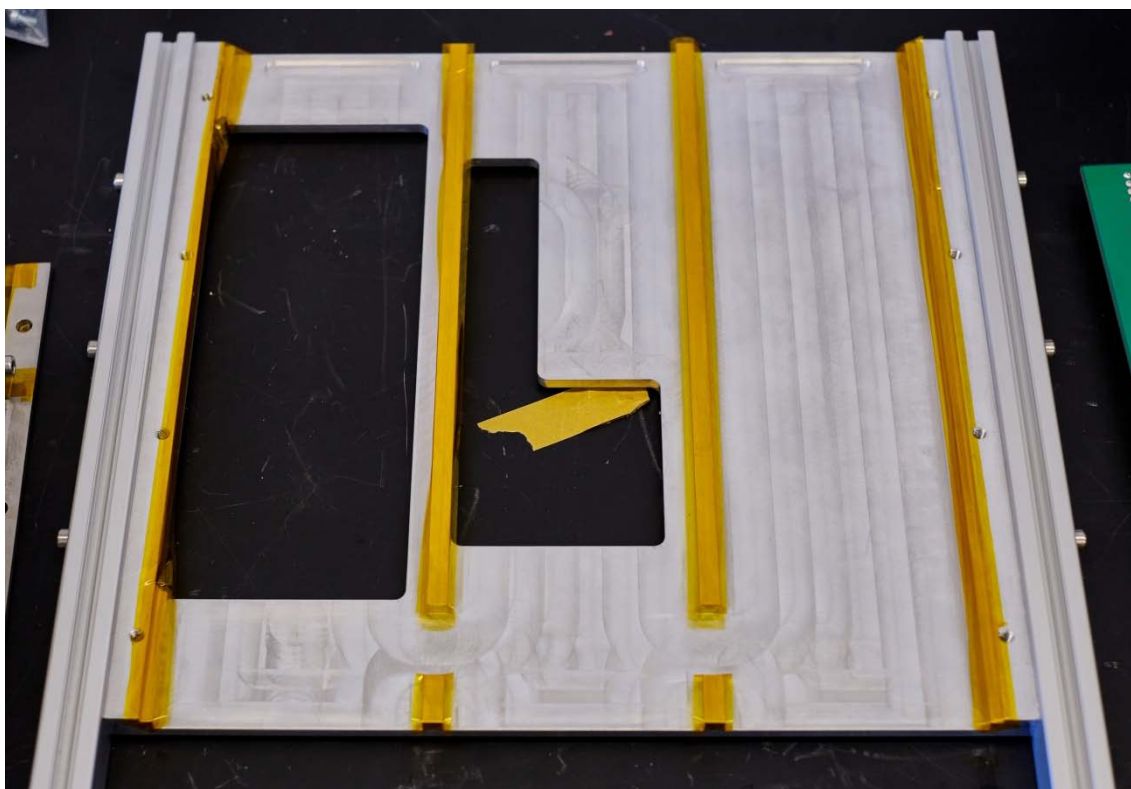
Figure 4.13 Pathfinder base plate with kapton [39]
