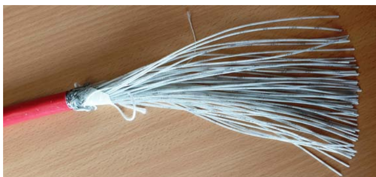
Figure 3.36 UT high voltage cable
