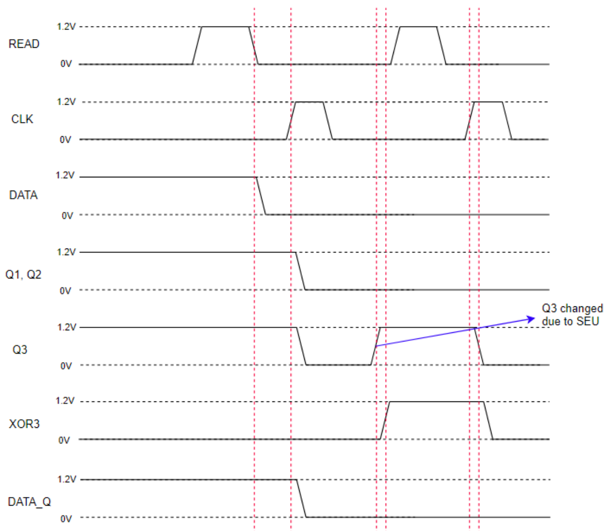
Figure 4.4: Internal signals in the core domain of the 1-bit eFuse cell. The DATA is read at the falling edge of the READ signal and stored as Q1, Q2 and Q3 at the rising edge of CLK. If there is a SEU at the output of the D-flip-flops, and for instance if it changes the value of Q3 (one of the stored outputs), XOR3 signal becomes logic high and it triggers additional READ and CLK signals. Since the final output DATA Q is the majority of Q1, Q2 and Q3, it is not affected by SEU.
