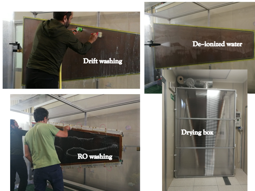
Figure 4.35: Different steps of the cleaning procedure. Drift panels are washed with NGL and Readout panel with CIF. Both are rinsed before with hot tap water and then with de-ionised water. Finally the washed panels are put in the drying box at 40°.
