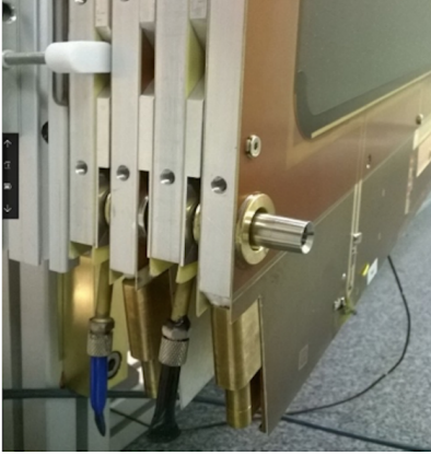
(a) Alignment Pin (installed on the Stereo panel) inserted in the pin slot (installed on the Eta panel).
