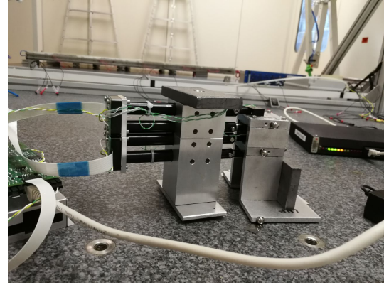
(b) 4-Rasfork during the calibration step at LNF using the Calirasfork.
