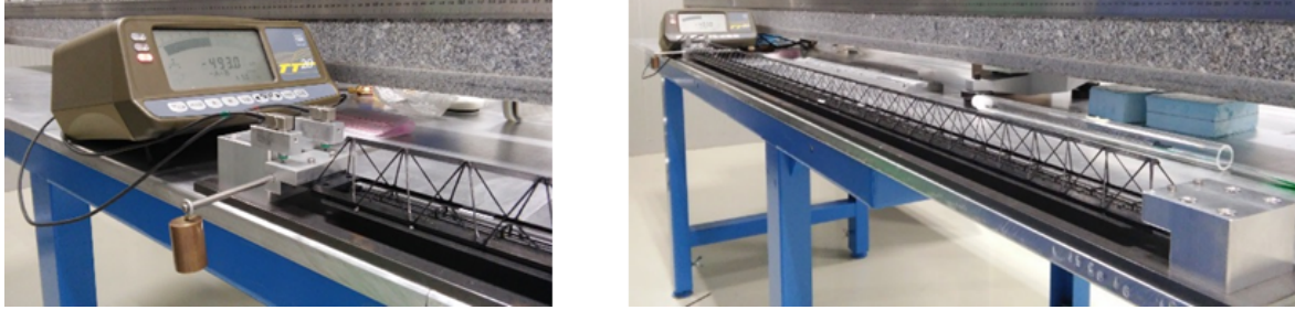
Figure 3.42: OB torsional test, set up.
