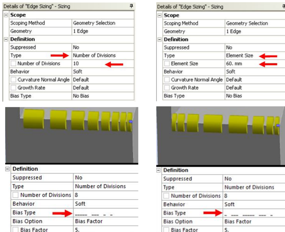
Figure B.3: Sizing controls. Growth Rate = Bias Factor n^{-1} , with n number of divisions.
