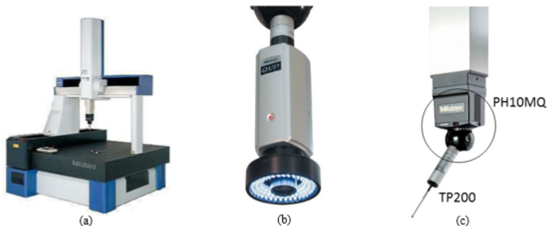
Figure 2.25: The Mitutoyo tools for assembly and metrological survey.
