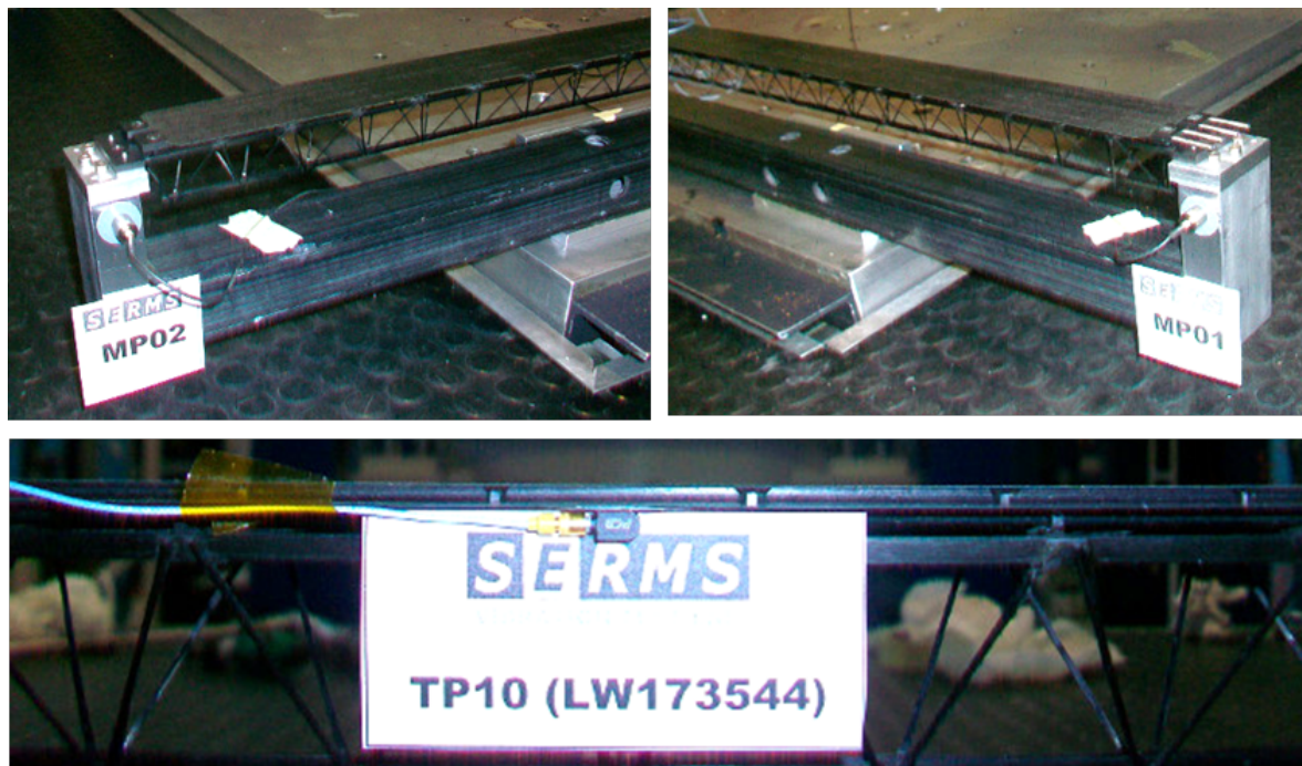
Figure 3.43: OB Stave vibration test, accelerometers set up.
