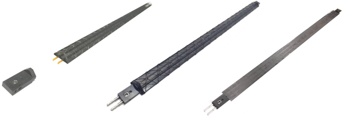
Figure 3.9: IB Stave prototype.
