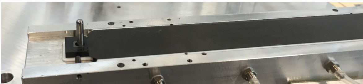
Figure 2.9: Cold Plate in position; with vacuum and dowel pin of H1.
