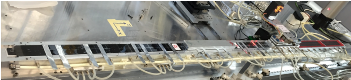
Figure 2.8: Half-Stave during assembly using dummies modules
