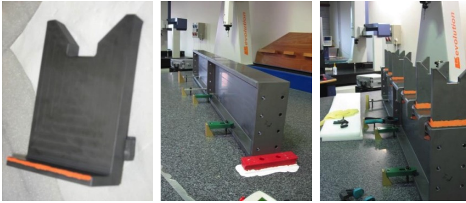
Figure 4-14: Case A monolithic parts made of SiC
