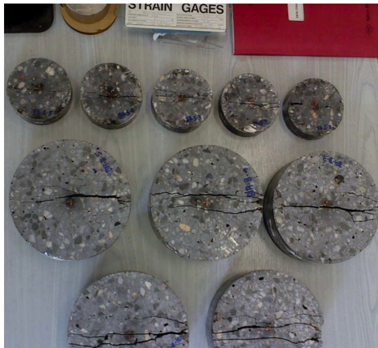
Figure 6-39: Epument samples after the Brazilian disc tests
