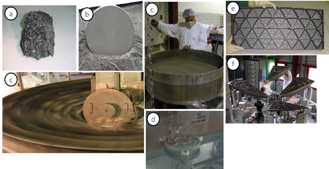
Figure 4-11: a) SiC raw material in grain, b) SiC powder and SiC monolithic component produced by sintering, c) Different phases of fabrication, d) Grinding of SiC component, e) SiC part during fabrication step, f) SiC parts of Herschel telescope in final assembly
