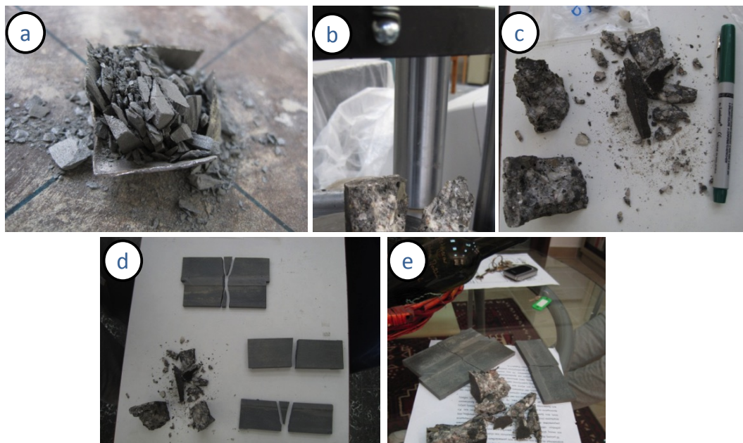
Figure 6-40: Specimens after testing a, b, c) UCT specimens, d, e) 3PB specimens.
