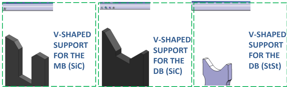
Figure 3-14: V-shaped support models for the MB and DB
