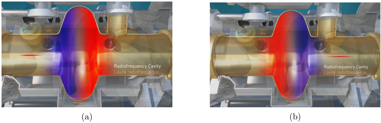
Figure A.1: RF cavity. The beam of particles is represented by a horizontal line in red. The electric fields are generated inside the cavity. The direction of the field oscillates according to the arrival of the particles. The red colour represents positive voltage, while blue represents negative voltage. (a) The protons feel attracted by the electric field when they are approaching the cavity. (b) The field changes polarity once the particles have traversed the cavity, repelling them and pushing them forwards along the beam pipes [35].
