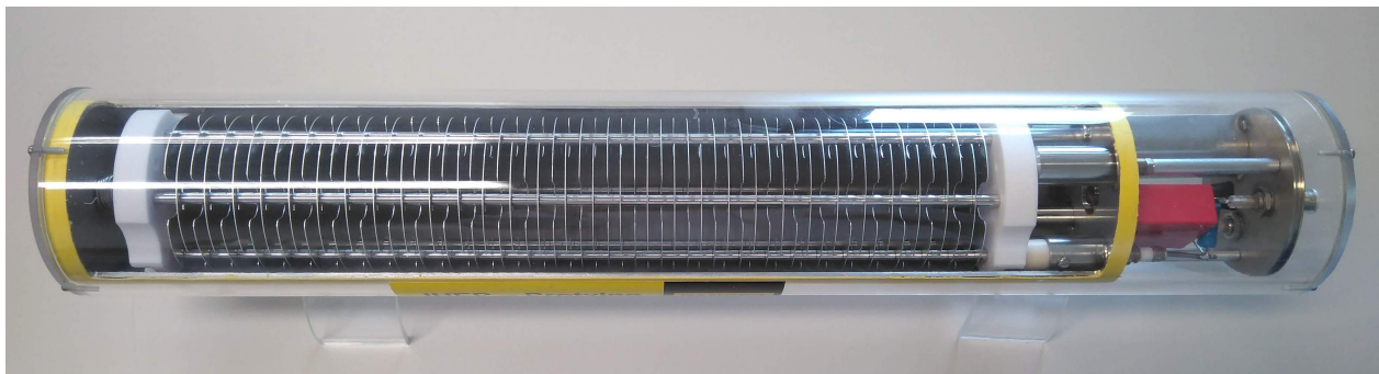
Figure 5: Internal part of an IC BLM showing the electrodes. The cables to the read-out electronics are located on the right part.
