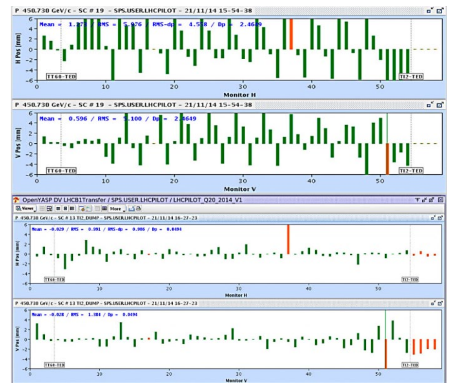
The upper plot shows the trajectory of the first T12 beam, which reached the end of the transfer line in a single attempt after 18 months of technical stop. Below, a smoother beam trajectory in T12 after some corrections.
