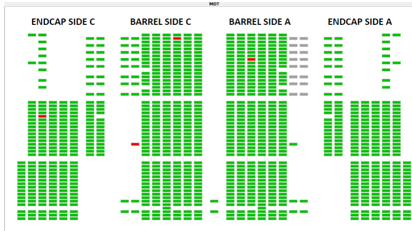
FIGURE 3.10: Screenshot of the MDT DQMD available in ATLAS Control Room since Run 3. The screenshot shows events from 13.6 TeV pp collision, run number 364292.
