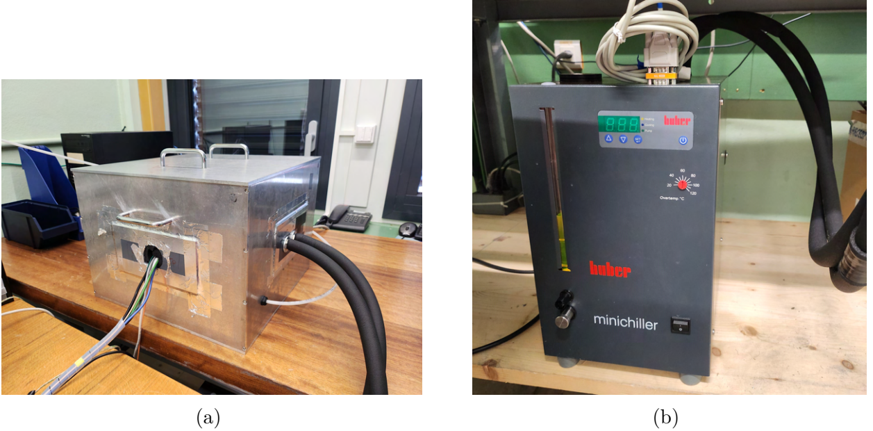
Figure 4.1: Picture of the thermally insulated, air-tight container (a) and the Huber Minichiller (b).
