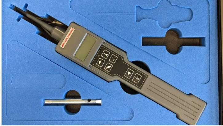
Figure 3.12: GasCheck G3 leak detector used to check for CO 2 leaks.
