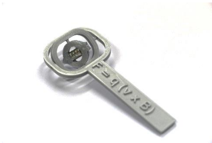
Figure 6. 3D magnetic compass printed as part of the project.
