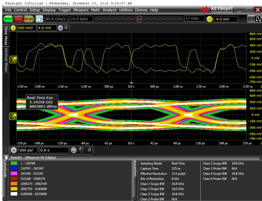
Figure 12.12: An eye diagram for DCB, produced overnight. Wide-open and has no noise in the eye, an indication of good signal quality.
