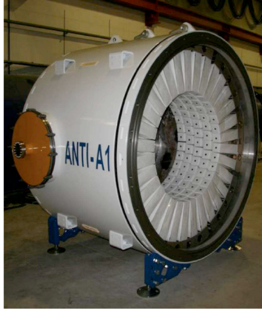
Figure 2.16: A module from the OPAL calorimeter (left). The 1st LAV station with 32 \times 5 wrapped OPAL lead glass calorimeter elements (right).
