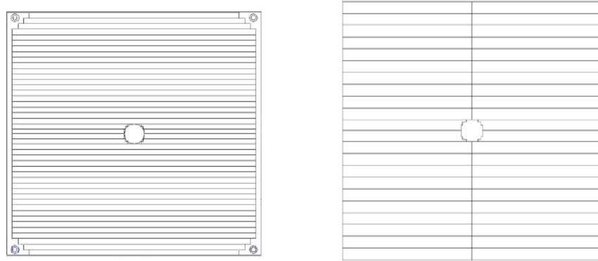
Figure 2.12: Layout of one scintillator layer of the MUV1 (left) and of the MUV2 (right)
