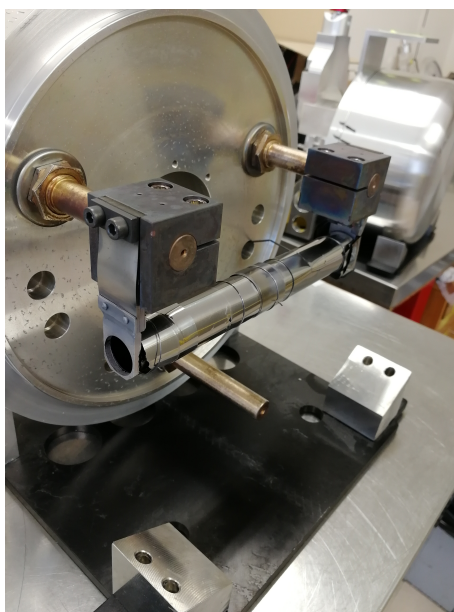
Figure B.1: Formerly applied ISOLDE heating unit, comprising a cylindrical Ta target container, Ta heat screen and copper blocks holding the assembly.
