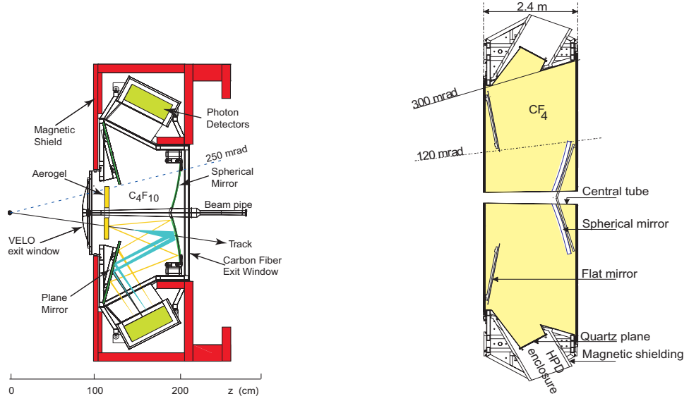
Figure 2.11: RICH1 (left) and RICH2 (right) detectors layout.
