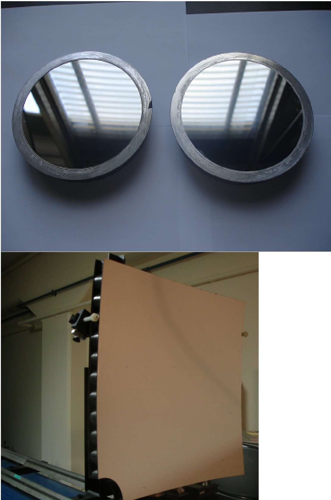
Figure 4.10: The mirrors used for the aging tests. Above are mirrors CMA1 and CMA2, below is the demonstrator mirror.
