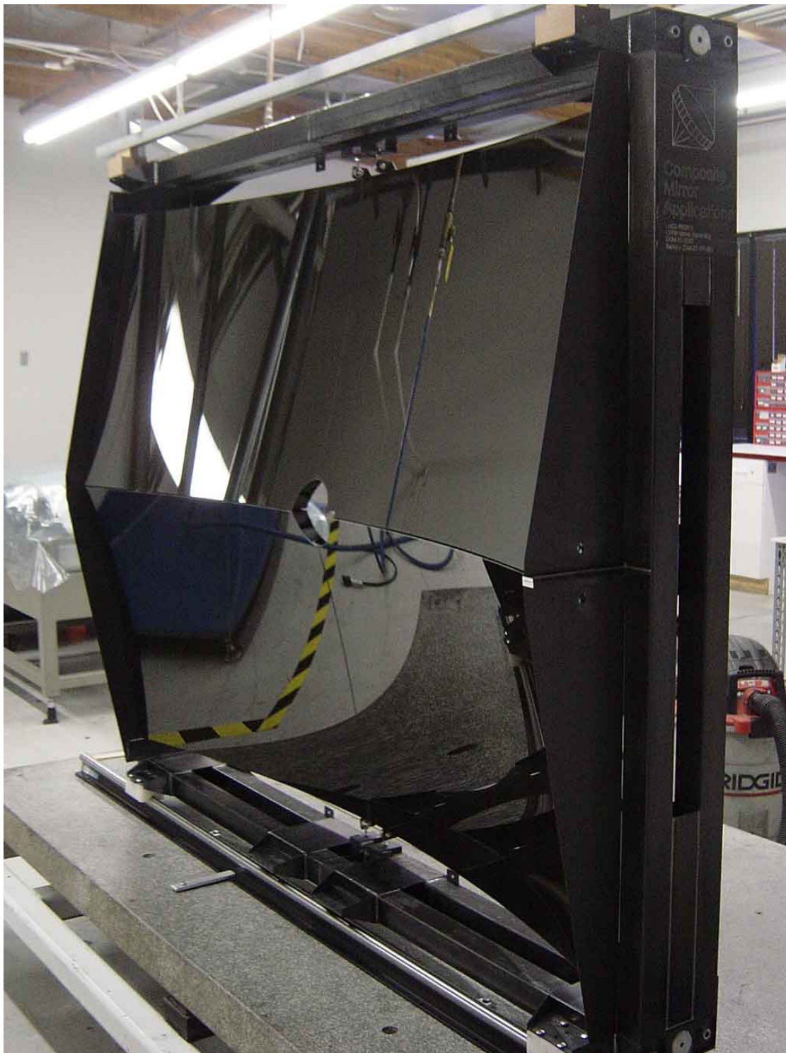
Figure 4.19: The RICH 1 spherical mirrors prior to coating by SESO
