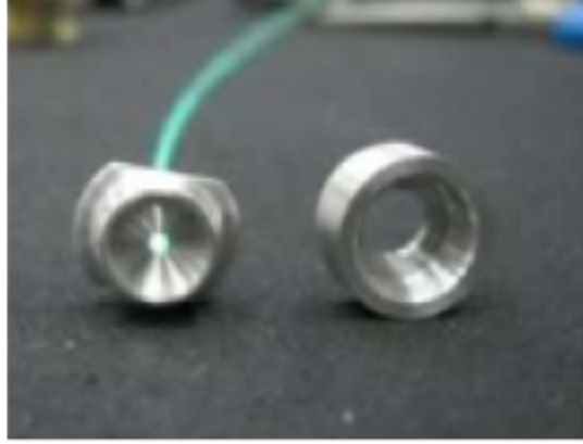
Figure 3.8: Fiber glued to the SiPM housing connector.
