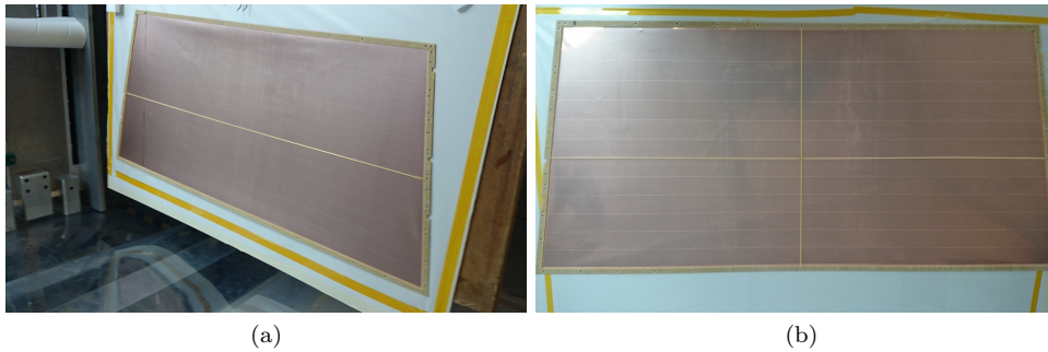
Figure 8.3: Bottom side of a framed OROC3 GEM foil. In (a), one bar is added to the frame while, in (b), two bars form a cross. In the latter configuration no foil sagging is visible any-more.
