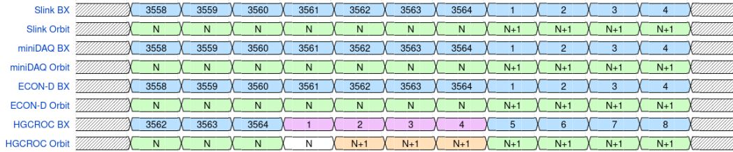
Figure 6.55: The wave diagram above shows the BX and Orbit counters for Slink, miniDAQ, ECON-D, and HGCROC, highlighting the artifacts in the BX and Orbit counters caused by HGCROC V3 design flaws, indicated by magenta and empty boxes. Here N is the current Orbit count and N + 1 is the incremented Orbit count.
