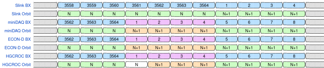
Figure 6.56: The wave diagram above shows the BX and Orbit counters for Slink, miniDAQ, ECON-D, and HGCROC in the actual test setup, where miniDAQ and ECON-D's BX counters have an offset of 4 to align with HGCROC's BX counter. The empty box highlights that the Orbit counter of HGCROC does not increment correctly at the BX rollover.
