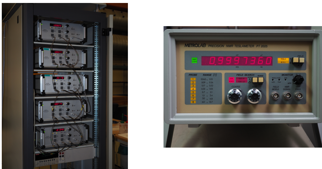
Figure 5.1: Left: Portable Digital Integrators (PDI) in their rack. Right: Nuclear Magnetic Resonance (NMR) device
