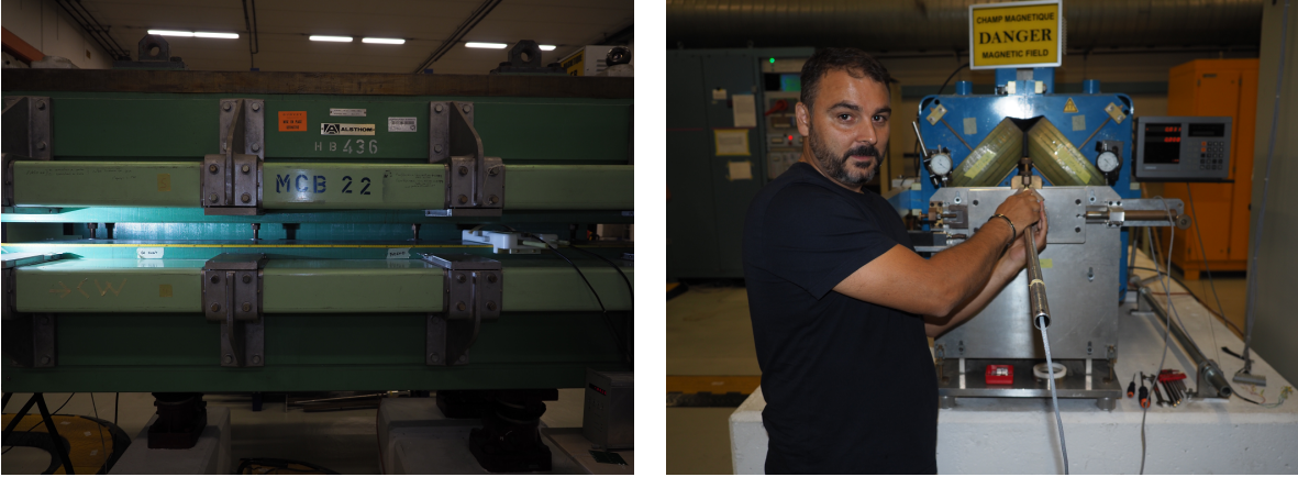
Figure 3.3: Left: Dipole reference magnet. Right: Quadrupole reference magnet with installed equipment for radius calibration operated by the head of the technicians associated to the MM section.
