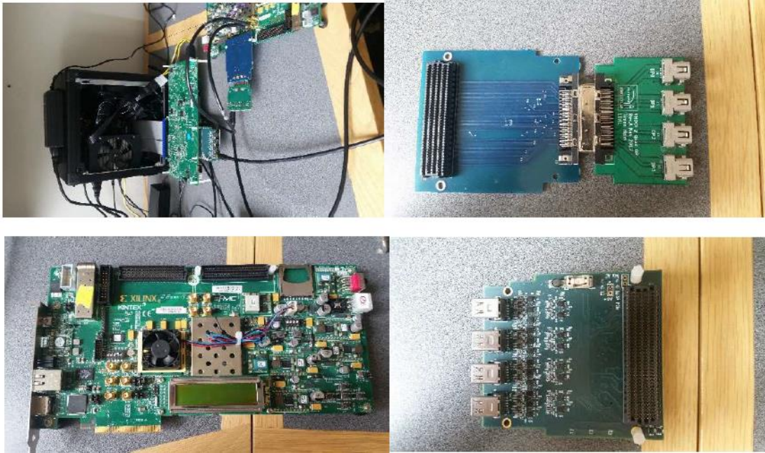
Figure 22: Top left: YARR setup at UW. Top right: FMC to DP breakout board. Bottom left: KC705 Xilinx board. Bottom right: Ohio MMC card [13]
