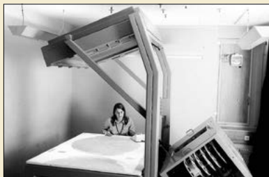
A prototype of BESSY, the scanning table designed specifically for use on film from BEBC, delivered to CERN in December 1971. (Image credit: CERN-EX-7204071.)
