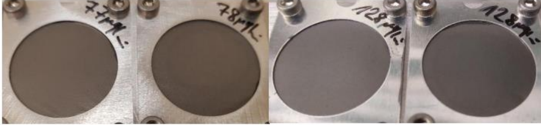
Figure 8: Stripper foils with different thicknesses (77, 78, 128, and 128 \mu\text{g}/\text{cm}^2 )
