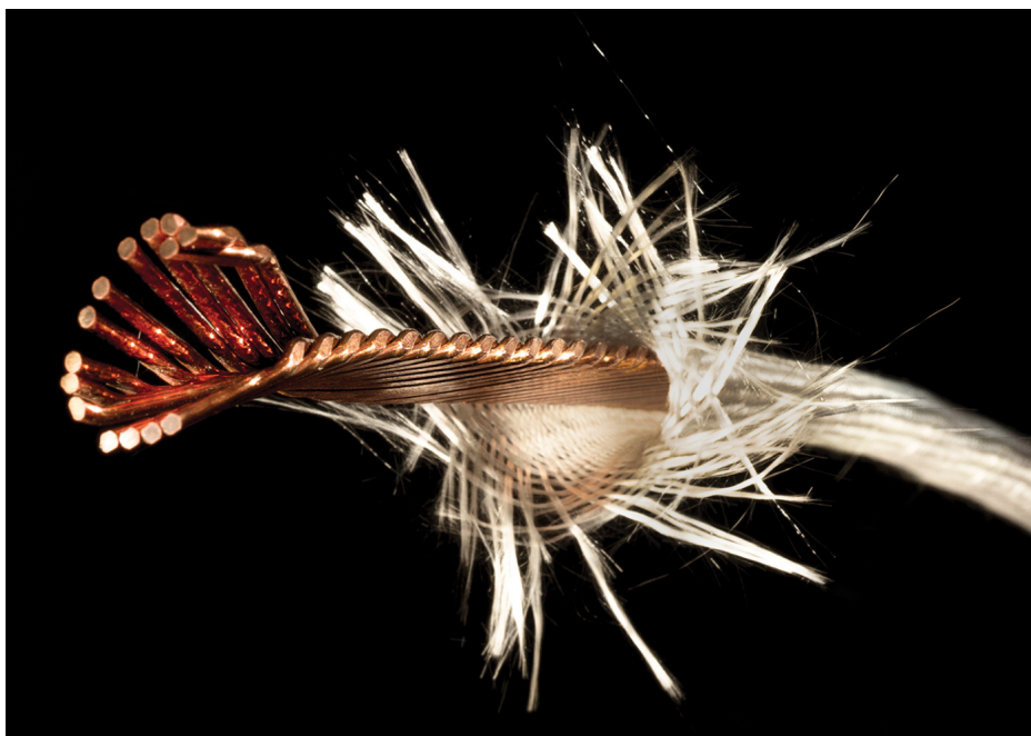
A niobium-tin cable (Nb 3 SN), showing the single strands, partially unwrapped (Image: Maximilien Brice/CERN)
