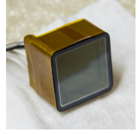
Figure 8: Photo of the MCP-PMT [1]. It is a miniPLANACON type from Photonics [6] .
