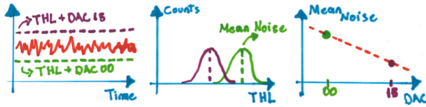
Figure 6.14: Steps taken during the equalisation of a single pixel. On the left a single pixel has a particular noise level, the threshold can be altered by setting a local 4-bit DAC (between 00 and 15). On the centre, if the global threshold is varied with a fixed local threshold, one can find the DAC value with maximum noise counts. By scanning the global threshold with the two extreme value of the local threshold, one can parametrise how the maximum number of noise counts varies with the local DAC. The equalisation then tries to minimise the variance on the position of the noise for all pixels by setting the local threshold accordingly.
