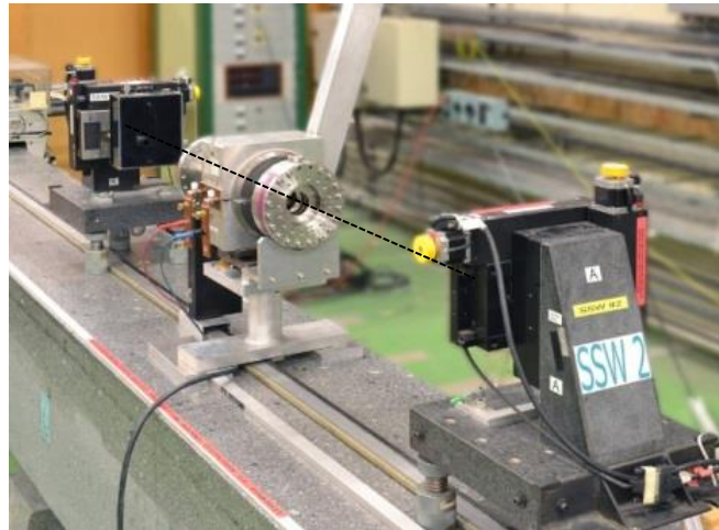
Figure 9: Example of stretched wire metrology system used for fitting a wire to components electrical or magnetic axis or for studying the field quality (courtesy of CERN) (Arpaia et al. , 2015; Caiazza, 2015; Mainaud Durand et al. , 2016).
