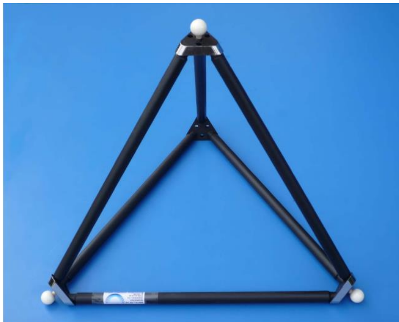
Figure 42: Carbon fibre tetrahedron artefact used for CMM uncertainty model validation (Trapet, 2017)
